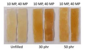
The appearance of unfilled and silica-filled samples with 10 and 40 milling passes.
