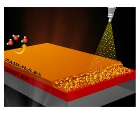
**Caption:** Researchers have developed a new precision spray-coating method called sequential spray deposition that enables multilayer perovskite absorber for advanced solar cell designs and could be scaled up for mass production. The technique could be used to create perovskite architectures with any number of layers.
